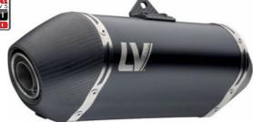
using a 2x2 twill weave carbon fibre that is pre-impregnated with a special high temperature resistant resin and then vacuum cured in a hot press. For optimised mechanical resistance and weight reduction, a carbon fibre bracket bolted to the muffler sleeve emphasises the clean lines and asymmetrical styling.
